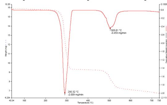
Fig. 5. The TG/DTA curve of BaCl<sub>2</sub> doped KHP.
