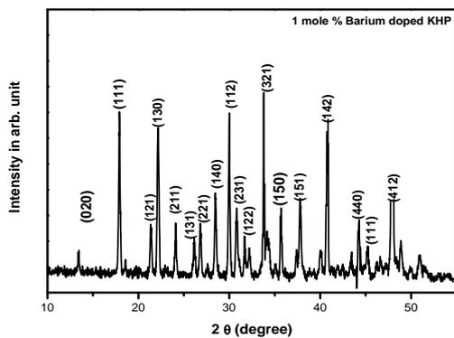
Fig. 2. Powder XRD pattern for BaCl<sub>2</sub> doped KHP.
