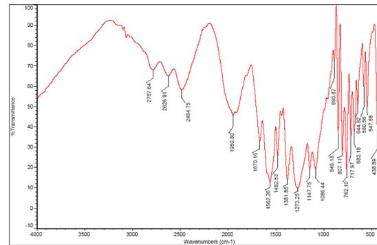
Fig. 4. The FTIR spectrum of BaCl<sub>2</sub> doped KHP.
