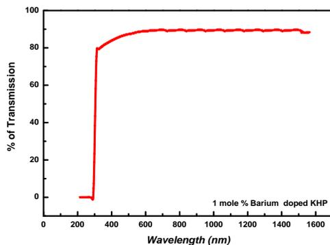
Fig. 3. The UV-Vis spectrum of BaCl<sub>2</sub> doped KHP.
